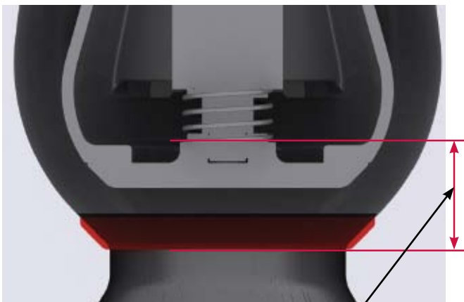
Short stroke, very low flow velocity to fully open the valve, short closure time.
